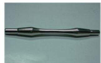
Fatigue test specimen
