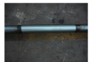
ND tested welded shaft
