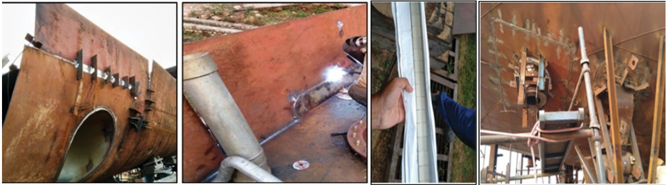
Ceramic Back-strip welding in Thruster Tunnel of Sagar Anveshika & Hull of Sagar Tara
