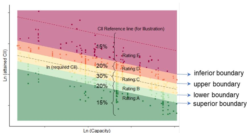
**Figure 1: Operational energy efficiency performance rating scale**
