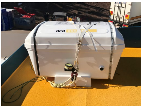
Correctly fitted HRU on a life raft
